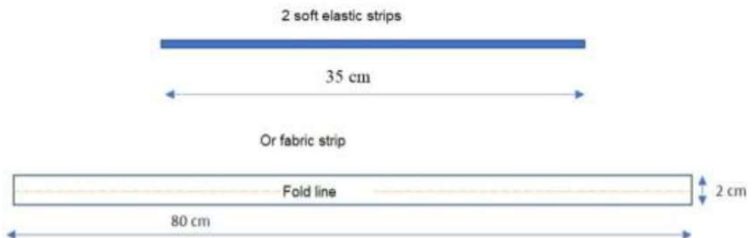
Figure 8 — Flat-fold - Sizing of the head harness
