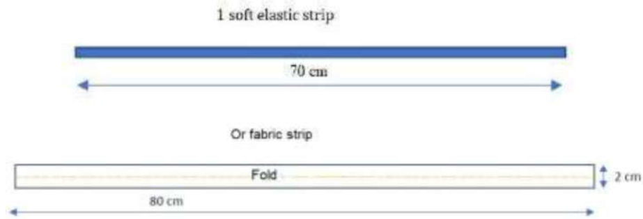
Figure 5 — Duckbill - Sizing of head harness
